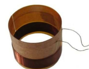
Moving coil for speaker 35-37mm ASV 2 Layers 40hm Characteristics Internal measurement: 35mm External measurement: 37mm ASV 2 Layers 4 ohms Winding height: 15mm Stand height: 38mm
