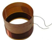
Moving speaker coil - 100mm 8Ohm Winding height: 21mm Support height: 55mm
