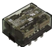
Relè 12V 4PDT - SP4-DC12V - NAIS Caratteristiche Mounting Type Through Hole Coil Voltage 12VDC Contact Form 4PDT (4 Form C) Contact Rating (Current) 10A Switching Voltage 250VAC, 30VDC - Max Coil Type Non Latching Features - Termination Style PC
