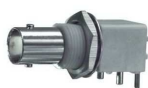
Connettore BNC Femmina da CS isolato Produttore : AMP P/N : 5227161-9 Connector Style BNC Connector Type Jack, Female Socket Contact Termination Solder Shield Termination Solder Impedance 50 Ohm Mounting Type Panel Mount, Bulkhead; Through
