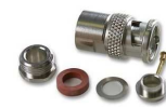
Coaxial Cable Types: RG59 Coaxial Termination: Solder Connector Body Style: Straight Plug Connector Mounting: Cable Connector Type: BNC Coaxial Contact Material: Brass Contact Plating: Gold Frequency Max: 1.5GHz Impedance: 75ohm SVHC:
